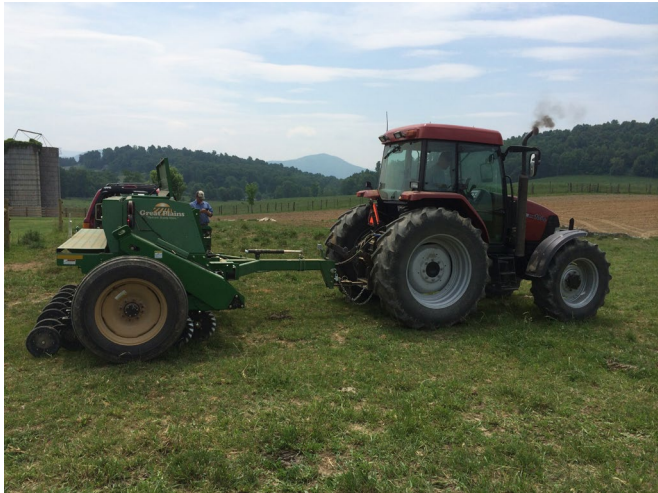
Figure 3. Seeding using a no-till drill. Photo provided by Cory Guilliams, Natural Resources Conservation Service.
