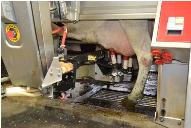
Figure 1. Automatic milking system in use.
